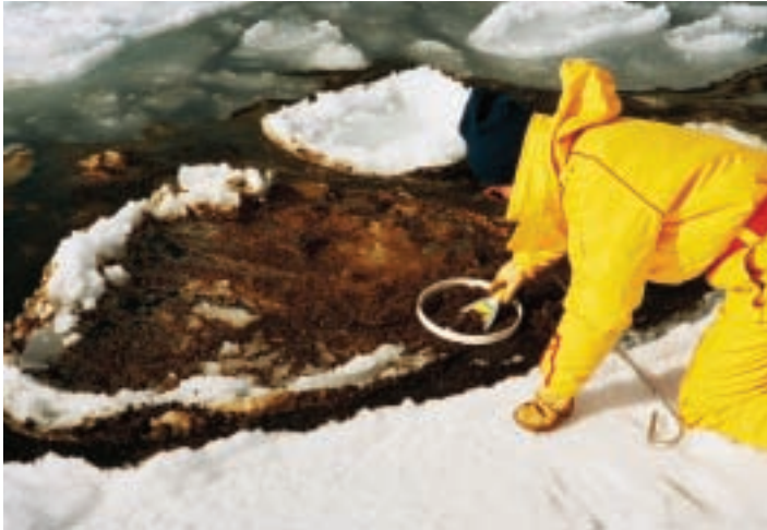
Sampling oil on the surface of pancake ice during an experimental spill in pack ice off Nova Scotia, Canada in 1986 (Ref. SL Ross and DF Dickins, 1987)
