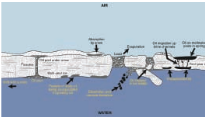
Schematic showing a number of possible configurations of oil in sea ice. Note that there is no multi-year ice off Sakhalin (Bobra and Fingas, 1986)
