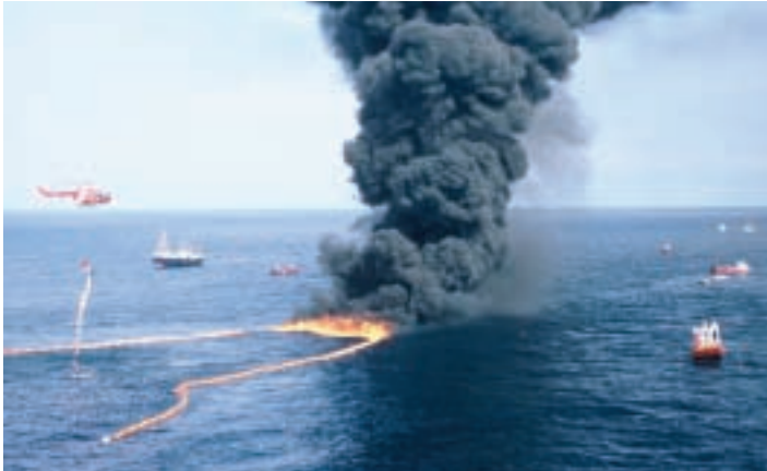
Helitorch being used to ignite oil contained in a fireproof boom during an Experimental spill offshore Newfoundland in 1993. Photo: Environment Canada
