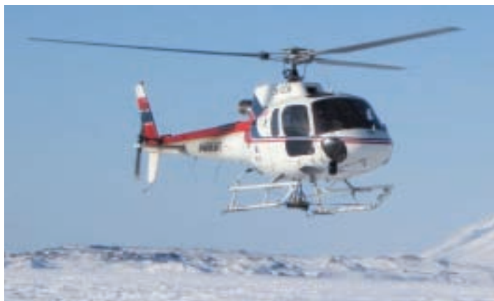
16. Helicopter flying a suspended ground penetrating radar over an experimental spill under sea ice in Norway, March 2006 (Photo: D. Dickins)
