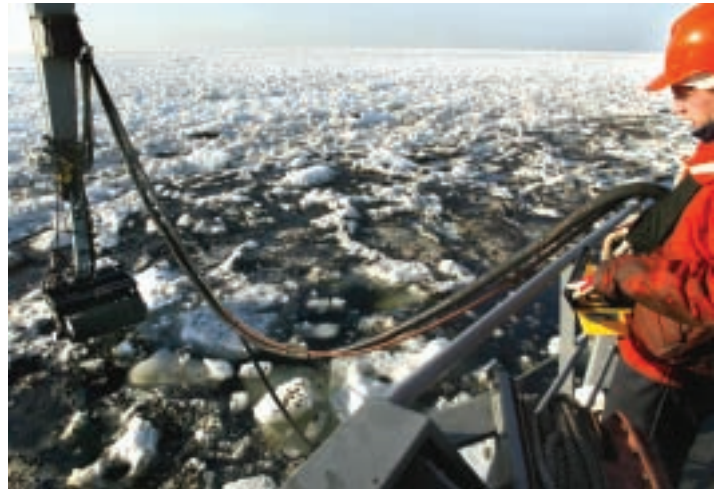
Brush bucket combination skimmer being used over the side of an oil spill response vessel to recover oil on ice during an accidental spill in the Baltic. Photo: Finnish Environment Institute
