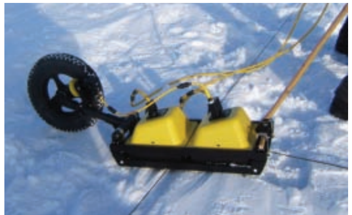
Boise State University scientists towing a portable ground penetrating radar system over oil trapped under under ice during an experimental spill in Norway, March 2006 (Photo: D. Dickins)
