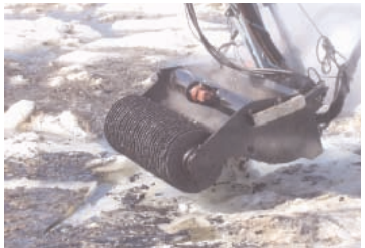
Brush bucket combination skimmer (close up). Photo: Finnish Environment Institute
