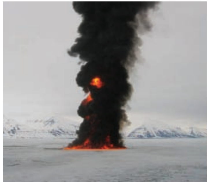
In-situ burning in late May 2006 of approximate 3000 litres of Statfjord crude spilled experimentally two months earlier under sea ice in Svalbard Norway. Burning time 11 minutes. Photo: SINTEF
