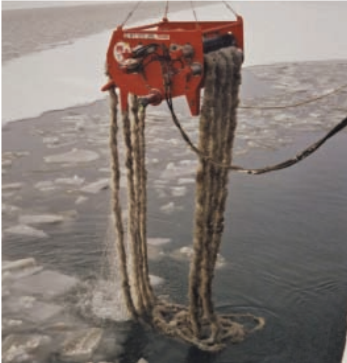
Rope-mop skimmer being demonstrated in broken ice in Alaska (Photo: Alaska Clean Seas)
