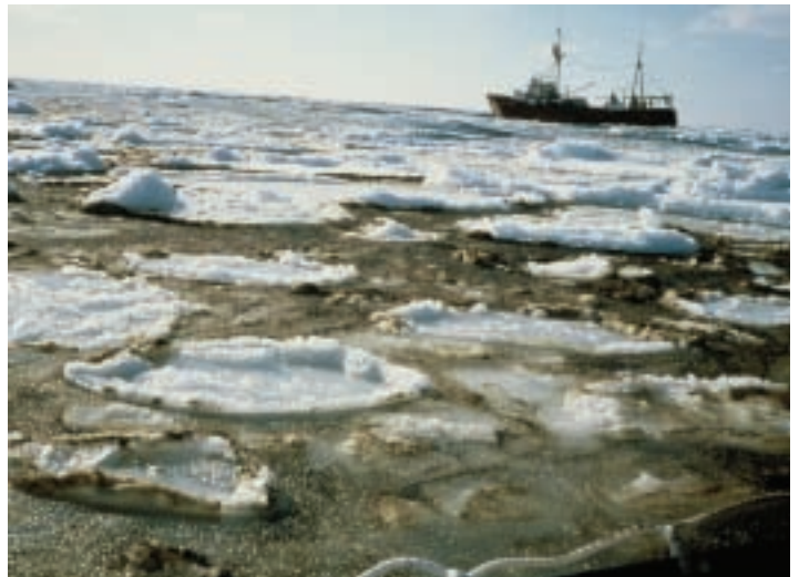
Oil in slush among pancake ice during an experimental spill in pack ice off the coast of Nova Scotia, Canada in March 1986 (Ref. SL Ross and DF Dickins, 1987)
