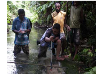
Figure 10 - Taking water flow measurements on the Talise River
